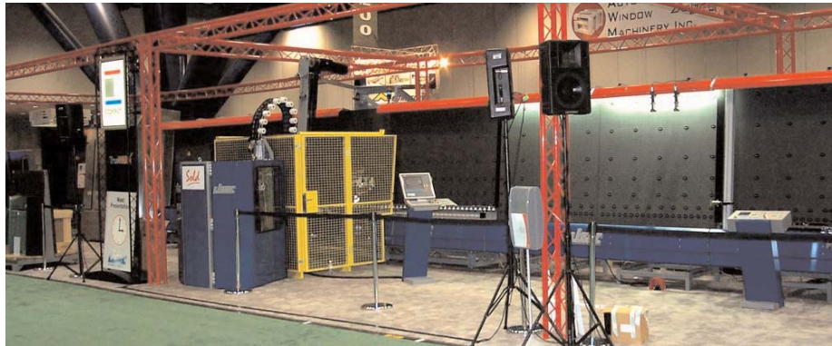
The Lisec-Edgetech True Warm Spacer System can produce up to 1200 units per shift with a cycle time of approximately 20 seconds.
