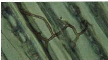
Fungal mycelia inside wood cells causing soft rot
